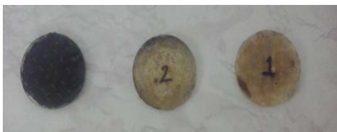
Fig. 3 Photograph of samples of composite materials used in Lee's disk.
